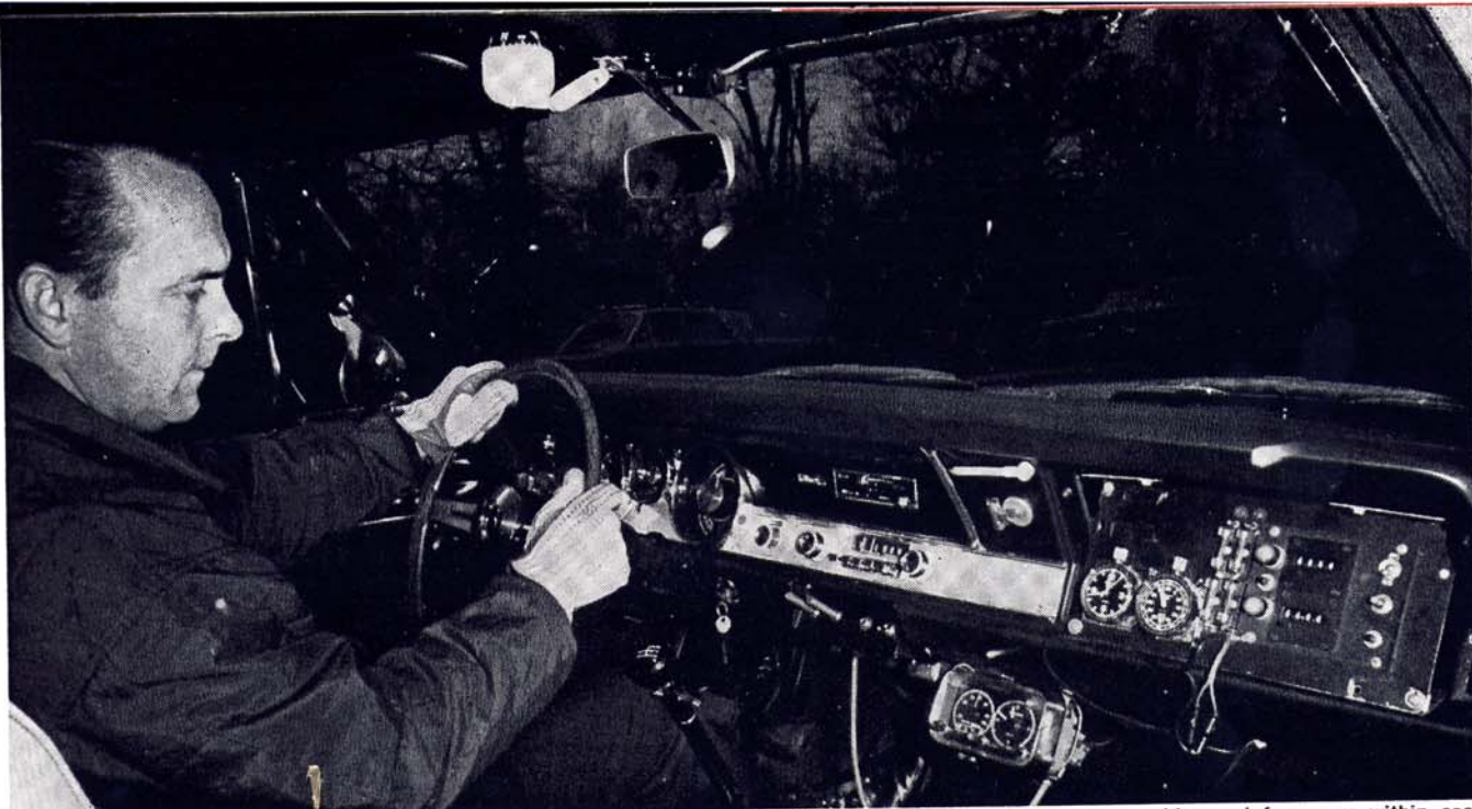
In the rally office, watches and odos replace the glove box, driving light switches replace the ashtray, extra cables and fuses are within easy reach. The Halda and compass are positioned so both of the crew can read them, and magnetic clips on the dash have unlimited purposes.
